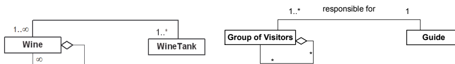
Figure 2 Representations of a Quantity (a-left) and a Collective (b-right) with their respective parts in UML conceptual Models.
