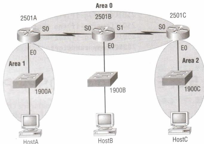
1. Configure the network between 2501A and 2501B and the Ethernet interface on 2501A. Assign serial 0 to Area 0 and Ethernet 0 to Area 1. (To understand the wildcard bits, please read Chapters 4 and 5 of the Sybex CCNP: Routing Study Guide.)
