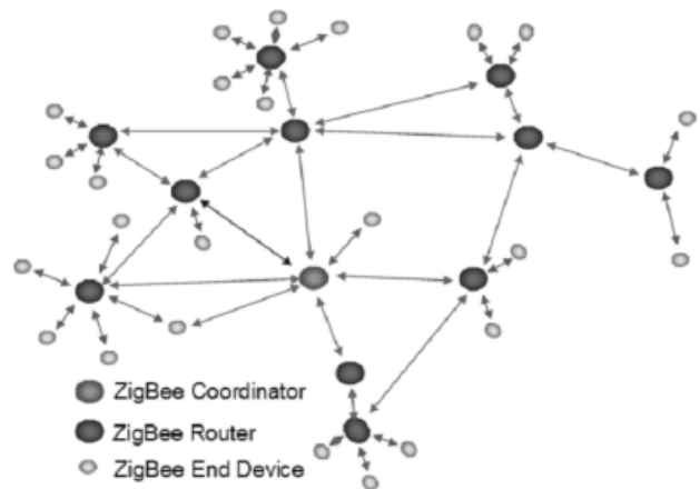
Figure 10. ZigBee Mesh Network and Device Types
